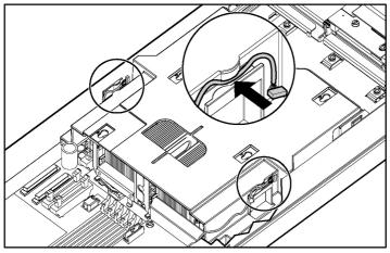
Figure 1-9: Attaching cables to the processor baffle
